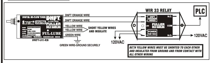
NOTE: DESCRIPTIONS OF RELAY CONTACTS GIVEN ARE BASED ON DNFT BEING IN OPERATIONAL MODE WITH LED "ON" THE WIR 33 RELAY.
